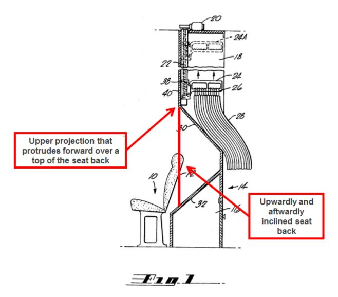
['742 Claim 12] The method of claim 11, wherein the upper projection is configured to abut an upper surface of the cabin area.
