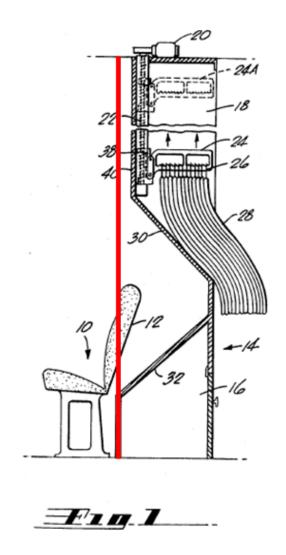
The Betts design therefore "reduc[es] or eliminate[es] gaps that existed between the previously-installed forward wall and the passenger seat."
