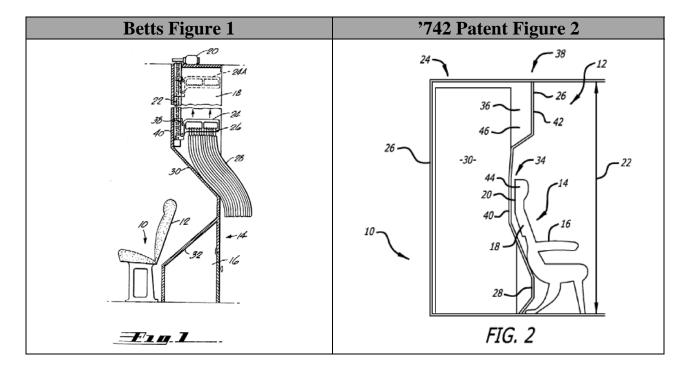
As explained above, a person of ordinary skill in the art would be motivated to modify a flat wall lavatory to use the Betts design on the forward wall of a lavatory. Ex. 1004, ¶243. Such a design would "reduce[] a volume of unusable space in a cabin area of a passenger aircraft," under the broadest reasonable interpretation of this claim phrase. *Id.* For example, the seat in Betts is positioned such that it resides within the contour, as is shown by the annotated image below. *Id.*
