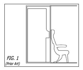
A person of ordinary skill in the art would realize that when such a seat is moved further aft, the first component to impact the wall is the seat back. Ex. 1004, ¶¶189-190, 250. As explained above, the KLM Crew Rest document shows a forward facing recess that receives the seat back when the seat is reclined. *Id*.
