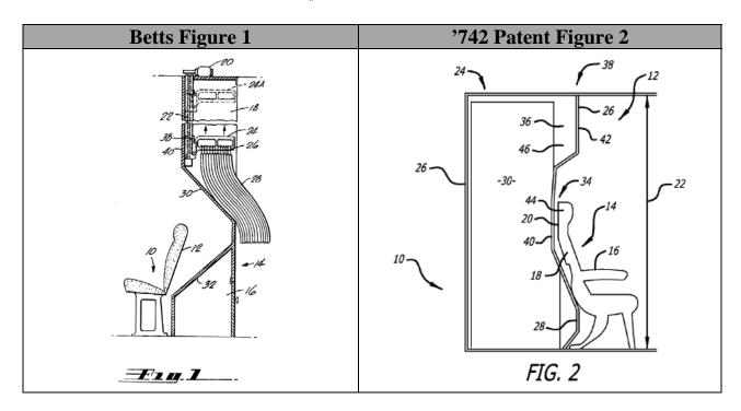
['742 Claim 8 Element B] the contoured forward partition comprises at least one first recess configured to receive at least a portion of an upwardly and aftwardly inclined seat back of a passenger seat therein, and
