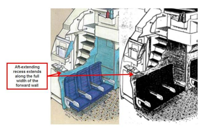
['742 Claim 16] The method of claim 8, wherein replacing the previously-installed forward partition with the contoured forward partition permits the aft-extending seat support to be positioned farther aft in the cabin area than was possible when the previously-installed forward partition was installed in the cabin area.
