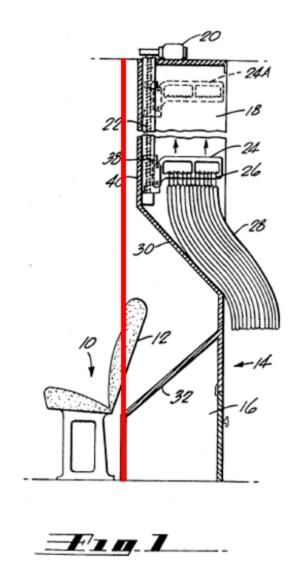
One of ordinary skill in the art would understand that the forward wall of the enclosure shown in Betts would also be suitable for use with other aircraft enclosures, including lavatories. Ex. 1004, ¶59. In an aircraft, as a row of seats is moved further aft, the first thing that makes contact with a flat wall is the top of the back of the seat. Ex. 1004, ¶59. And so Betts includes a recess that receives that portion of the seat back. Applying the contoured wall of Betts to a lavatory allows
