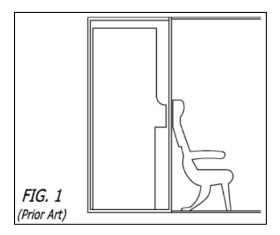
A person of ordinary skill in the art would realize that when such a seat is moved further aft, the first component to impact the wall is the seat back. Ex. 1004, Ex. 1004, ¶¶189, 250. As explained above, Betts includes a forward facing recess that receives the seat back. *Id*.
