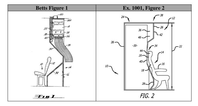
The Betts passenger seat has an exterior aft surface that is substantially not flat in a vertical plane. *See* Ex. 1005, Fig. 1; 2:7-14. Betts explains that this contour is positioned "to provide a space for seatback 12 to be tilted rearwardly." Ex. 1005, 2:19-24. One of ordinary skill in the art would understand that the coat closet includes walls forming a complete enclosure of the closet. Ex. 1004, ¶45.
