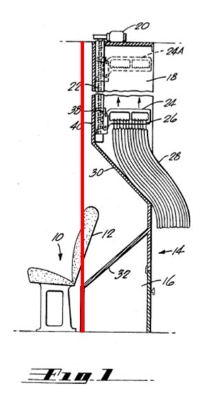
['742 Claim 8 Element A] replacing at least a previously-installed forward partition of a pre-existing aircraft lavatory in the cabin area of the passenger aircraft with a contoured forward partition, wherein an outward facing vertical surface of the previously installed forward partition is substantially flat, and
