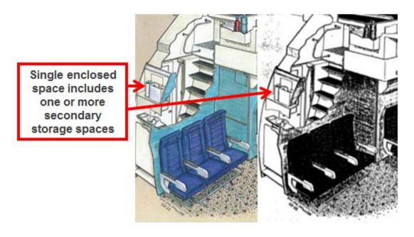
A person of ordinary skill in the art would understand that the enclosed space of a lavatory would continue to contain secondary storage spaces, such as amenity stowage, after applying a contour to the forward wall as shown by the KLM Crew Rest document. Ex. 1004, ¶207.
