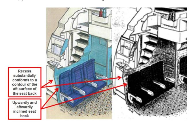
['742 Claim 11] The method of claim 8, wherein the contoured forward partition further comprises an upper projection that, upon installation, protrudes forward over a top of the upwardly and aftwardly inclined seat back.
