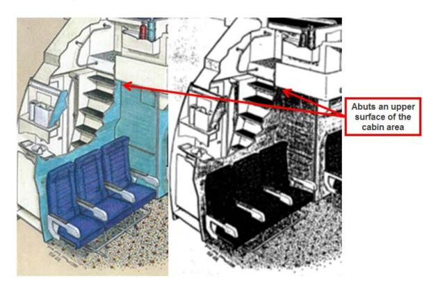
Further, the admitted prior art discloses a lavatory wherein the upper portion of the forward wall is configured to abut an upper surface of the cabin area.
