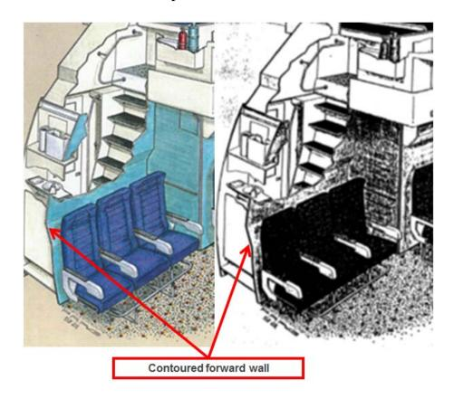
['742 Claim 8 Element B] the contoured forward partition comprises at least one first recess configured to receive at least a portion of an upwardly and aftwardly inclined seat back of a passenger seat therein, and
