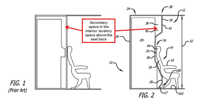
The KLM Crew Rest document also shows interior storage spaces within the enclosed lavatory space defined by the upper projection as shown in the annotated figure below. Ex. 1009; Ex. 1004, ¶111.
